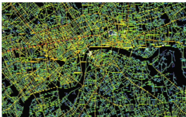
Figure 3 : Processed axial map of central London showing relative levels of spatial integration for all possible lines of pedestrian movement. Lines in warm colours are more spatially integrated, lines in cool colours less so.
