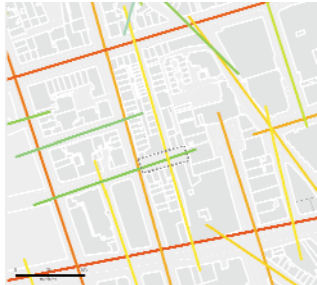
Figure 4 : Map of the area around St. Christopher's Place in central London (outlined in grey), showing lines of pedestrian movement. Lines in warm colours are more spatially integrated, lines in cool colours less so.
