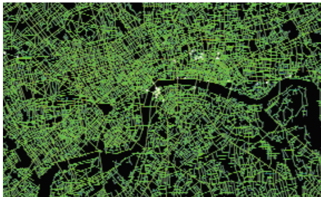
Figure 2 : Axial map of central London showing all possible lines of pedestrian movement.
